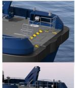
The active bow fender system reduces the impact forces to offshore structures and grants our clients a safe and smooth step over from and to offshore structures – even in bad weather conditions. In combination with the IPS propulsion system we aim at maximum uptime.
