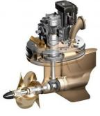
The new powerful propulsion system incl. 4 IPS thrusters delivering a fuel efficient drivetrain with perfect maneuverability including a joystick operated DP system.
